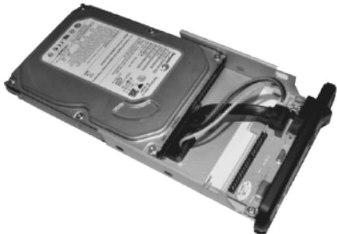
4. Fasten 4pcs screws to fix HDD.
